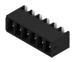
The SC-SMT pin header in 270°-outlet direction: the 270° angle exists between the plugging direction and the solder pin. The plugging direction is then parallel to the PCB. Sockets blocks, however, have an overhead plugging angle.
