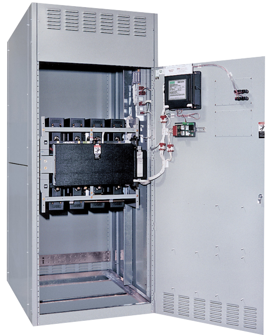
Fig. 3: Four pole, Delayed Transition 2000 Amp Transfer Switch.
