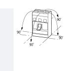
With XFI earth-fault release: - NZM1, N1, NZM2, N2: vertical and 90° in all directions
