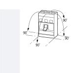
With XFI earth-fault release: - NZM1, N1, NZM2, N2: vertical and 90° in all directions
