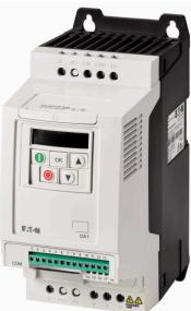
**Variable frequency drive, 230 V AC, 1-phase, 7 A, 1.5 kW, IP20/NEMA 0, Radio interference suppression filter, 7-digital display assembly**
