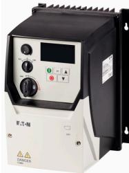
**Variable frequency drive, 230 V AC, 1-phase, 4.3 A, 0.75 kW, IP66/NEMA 4X, Radio interference suppression filter, OLED display, Local controls**
