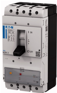
NZM3 PXR10 circuit breaker, 400A, 4p, variable, withdrawable unit
