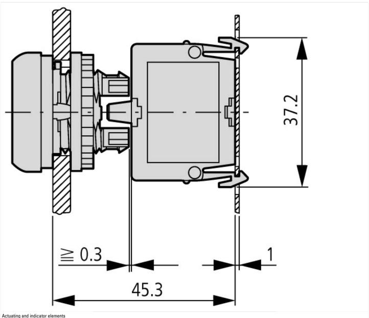
Actuating and indicator elements Base fixing
