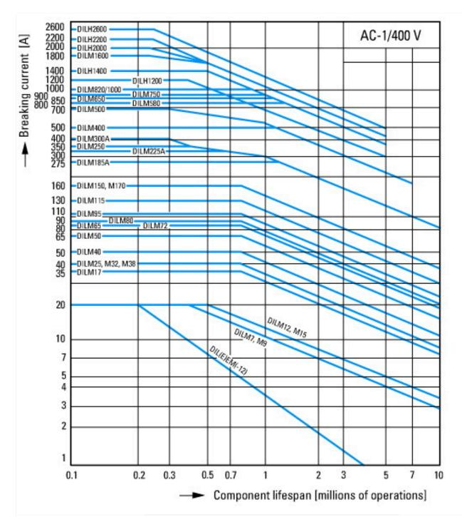
Switching conditions for non-motor consumers, 3 pole, 4 pole Operating characteristics
