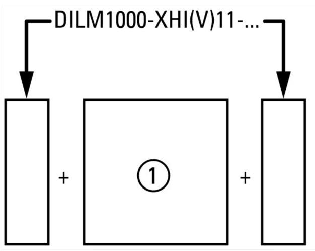
on the side: 2 x DILM1000-XHI(V)11-SI; surface mounting: 1 x DILM150-XHIA11 on the side: 2 x DILM1000-XHI(V)11-SA; surface mounting: 1 x DILM150-XHI (2 pole) on the side: 1 x DILM1000-XHI(V)11-SI; surface mounting: 1 x DILM150-XHIA22 on the side: 1 x DILM1000-XHI(V)11-SA; surface mounting: 1 x DILM150-XHI (4 pole)
