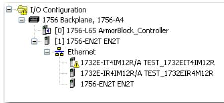
Warning signal – The module has a communications fault
