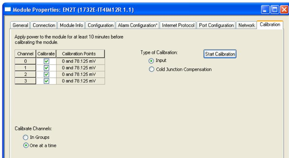
2. Check the Calibrate checkbox to specify which channel to calibrate.
