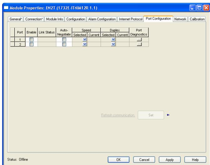
To configure the Ethernet ports, click the Port Configuration tab. This tab is only available for editing when the device is online.
