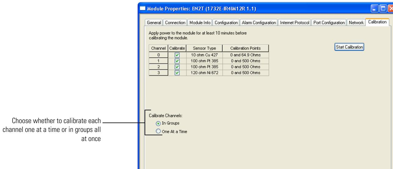
2. Check the Calibrate checkbox to specify which channel to calibrate.
