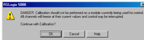
If at least one channel has been selected and there is a mismatch between the device in the RSLogix 5000 I/O Configuration and the actual physical device, another warning dialog comes up. It informs you that this is dangerous with an active system and there is a mismatch. This message box gives you an option to quit. Help is provided to you more information.
