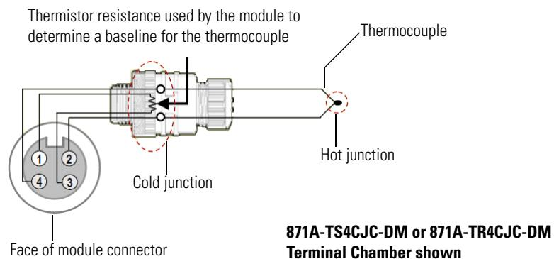
The compensation voltage to be applied can also be estimated by applying fixed cold junction correction using a fixed offset directly through the RSLogix 5000 software. The module supports thermistor compensation range at 0...70 °C.
