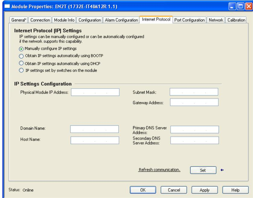
1. To configure your IP settings, click the Internet Protocol tab. This tab is only available for editing when the device is online. To manually configure your IP settings, specify the IP address in the Physical Module IP Address field.
