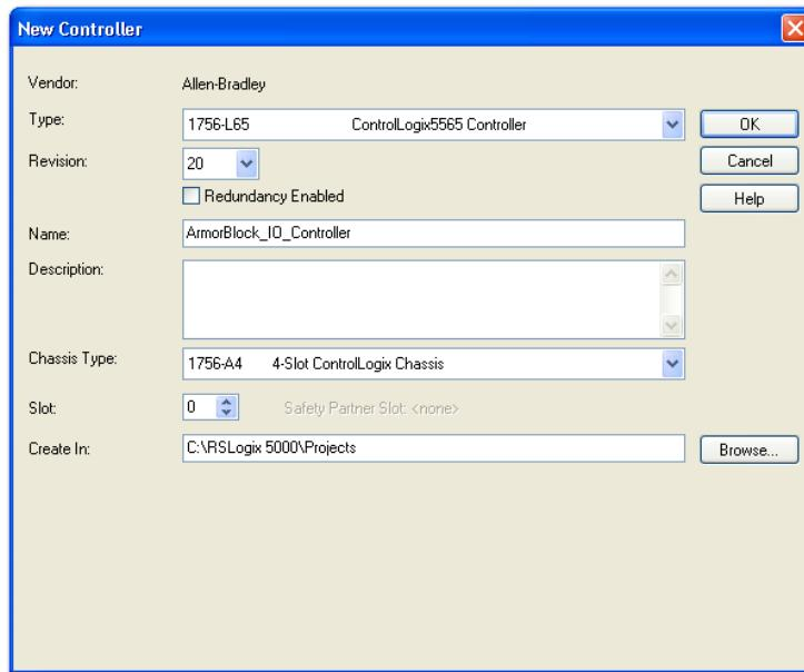
2. Enter an appropriate name for the Controller, for example, ArmorBlock\_IO\_Controller.
