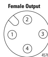
The power required by the module is based on a 4-pin micro-style connector system. Power can be daisy chained through the module either left to right or right to left. The standard configuration is with Module/Auxiliary power entering the module on the left connector.
