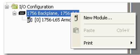
3. Expand Communications and select the new module in the Select Module dialog that appears. Select the 1756-EN2T EtherNet/IP Bridge.
