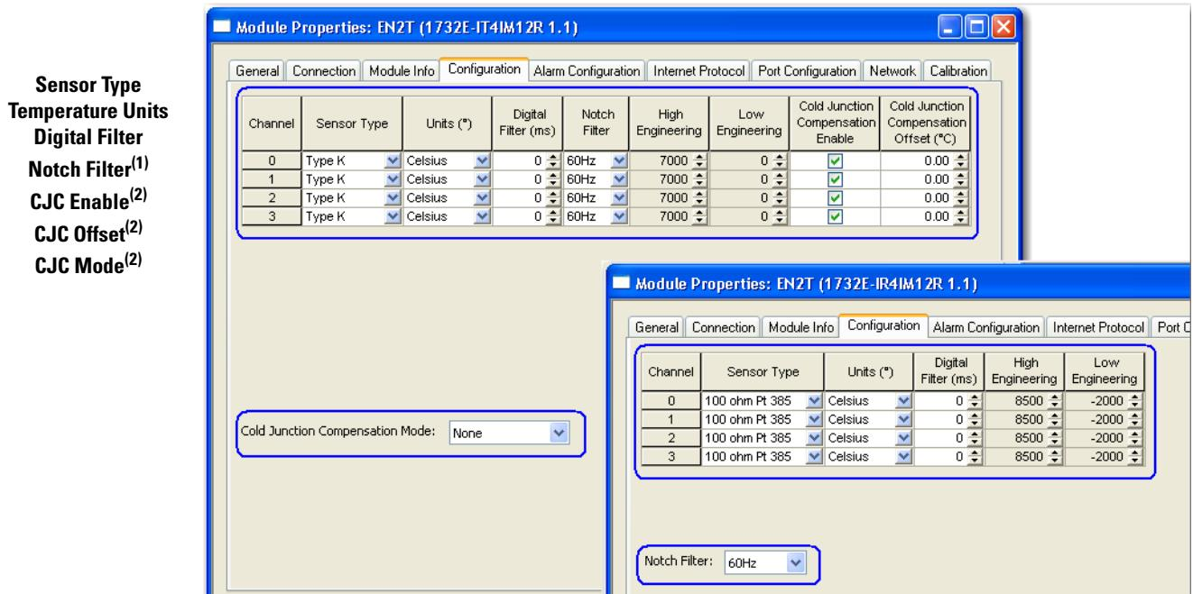
(1) Notch Filter can be set per channel on the Thermocouple module, and module-wide on the RTD module.
