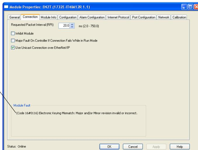
Status line provides information on the module fault and on the connection to the module
