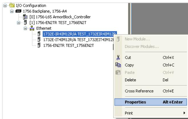
2. Select Properties. The Module Properties dialog appears and has the following tabs available for configuration.
