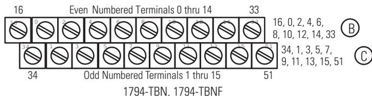
If continuing common to the next terminal base unit, connect a jumper from terminal 33 (24V DC common) on this base unit to terminal 16 on the next base unit.
