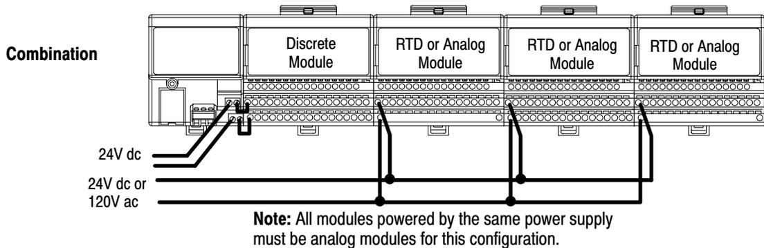
**Total current draw through any base unit must not be greater than 10A**
