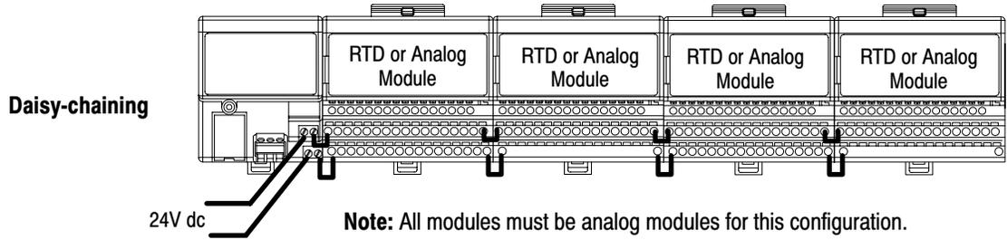
**Wiring when total current draw is less than 10A**
