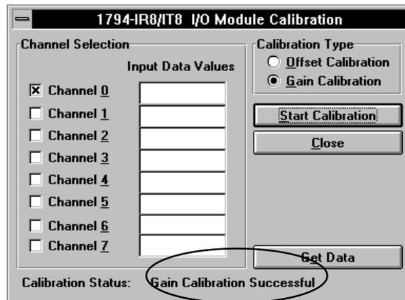
4. When calibration is complete, a notification will appear on the calibration status line.
