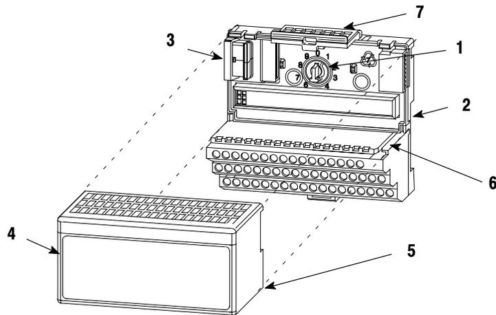
1. Rotate the keyswitch (1) on the terminal base unit (2) clockwise to position 3.
