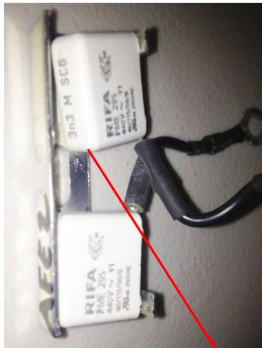
Close-up View of Common Mode Capacitor Assembly
