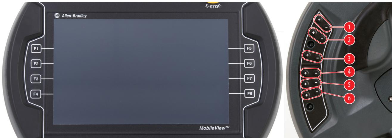
The keys on the MobileView 2711T terminal keypad operate similar to the keyboard of a Windows personal computer. Some 3-key combinations are supported. The following table shows the corresponding keyboard shortcut for each function key.
