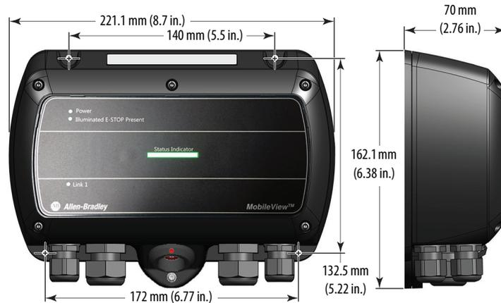
2. Use the back plate or the supplied cutout template to mark where to drill the four mounting holes for the junction box.
